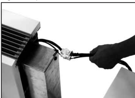
Fig. 57: Separate cable connectors
