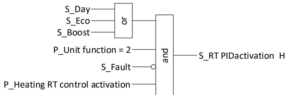
4.6.2.2 Cooling activation PID control algorithm
