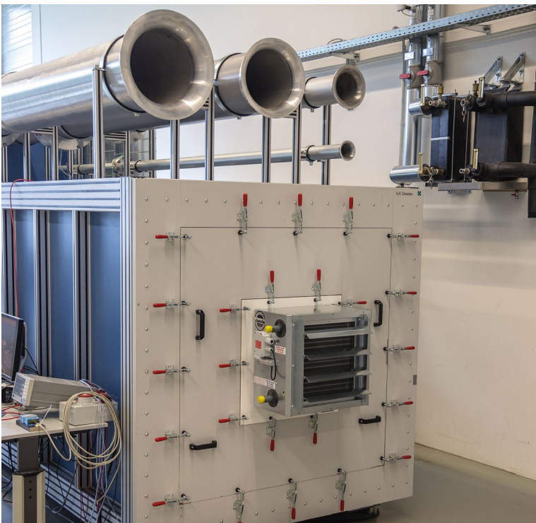
Test chamber for air performance measurements according to DIN EN ISO 5801, Kampmann R&D Centre
