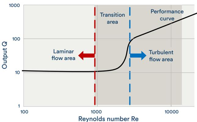
The diagrams clearly show the influence of laminar and turbulent flow on performance.
